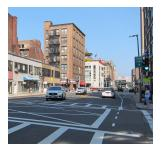
**Improved pedestrian visibility** by opening sight lines. Repainted crosswalks and "Don't Block the Box" markings. Modified the timing of WALK signals to give pedestrians a head start.
