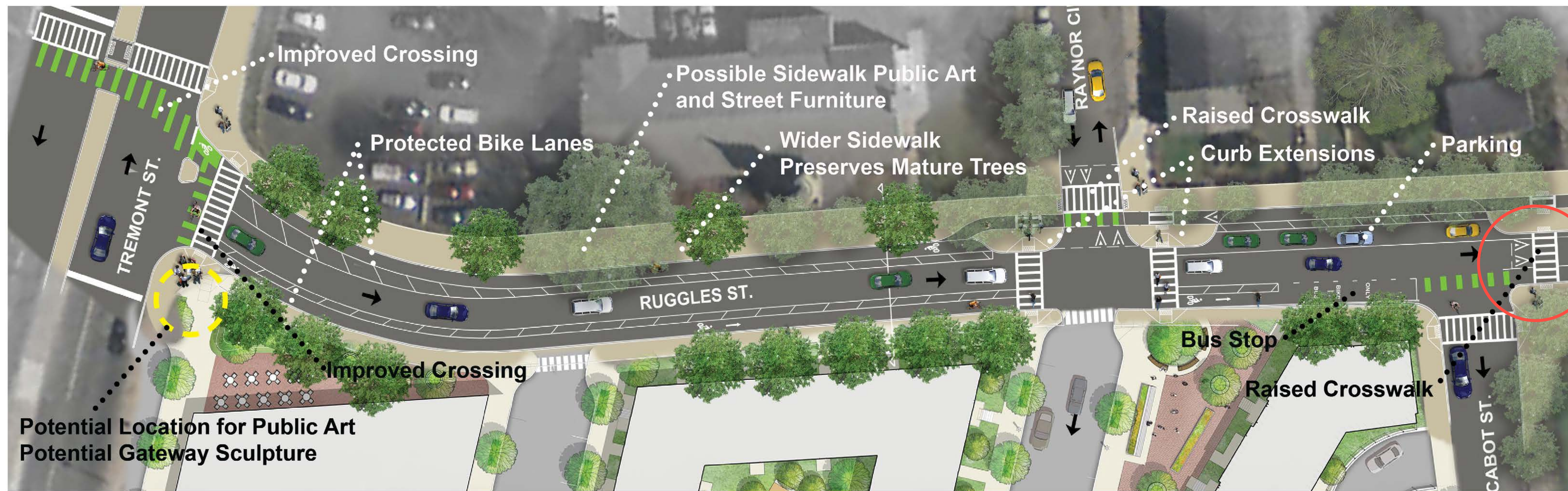
Proposed Improvements: Tighter curb radii, curb-extensions, raised crosswalks, lane delineation, ADA compliant sidewalks.
