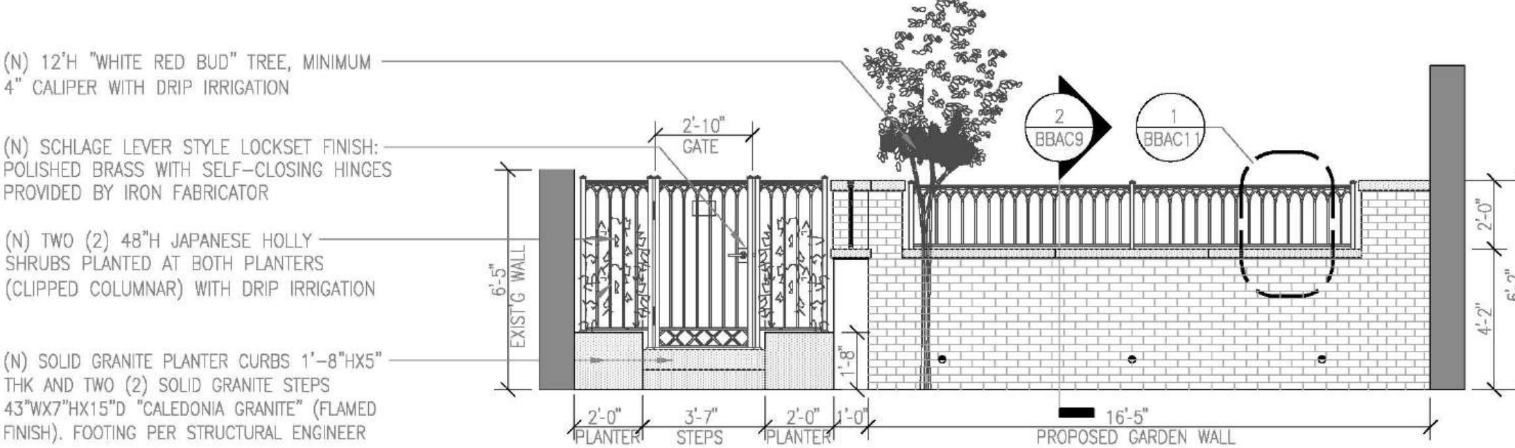
5 PROPOSED GARDEN WALL ELEVATION
