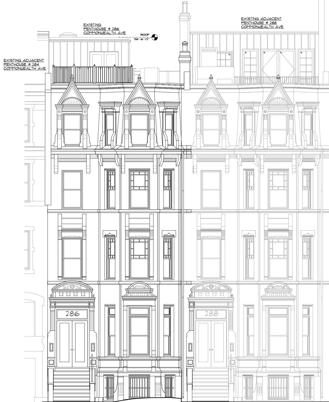
(E) EXISTING FRONT ELEVATION FULL: 1/4" = 1'-0", HALF: 1/8" = 1'-0"
