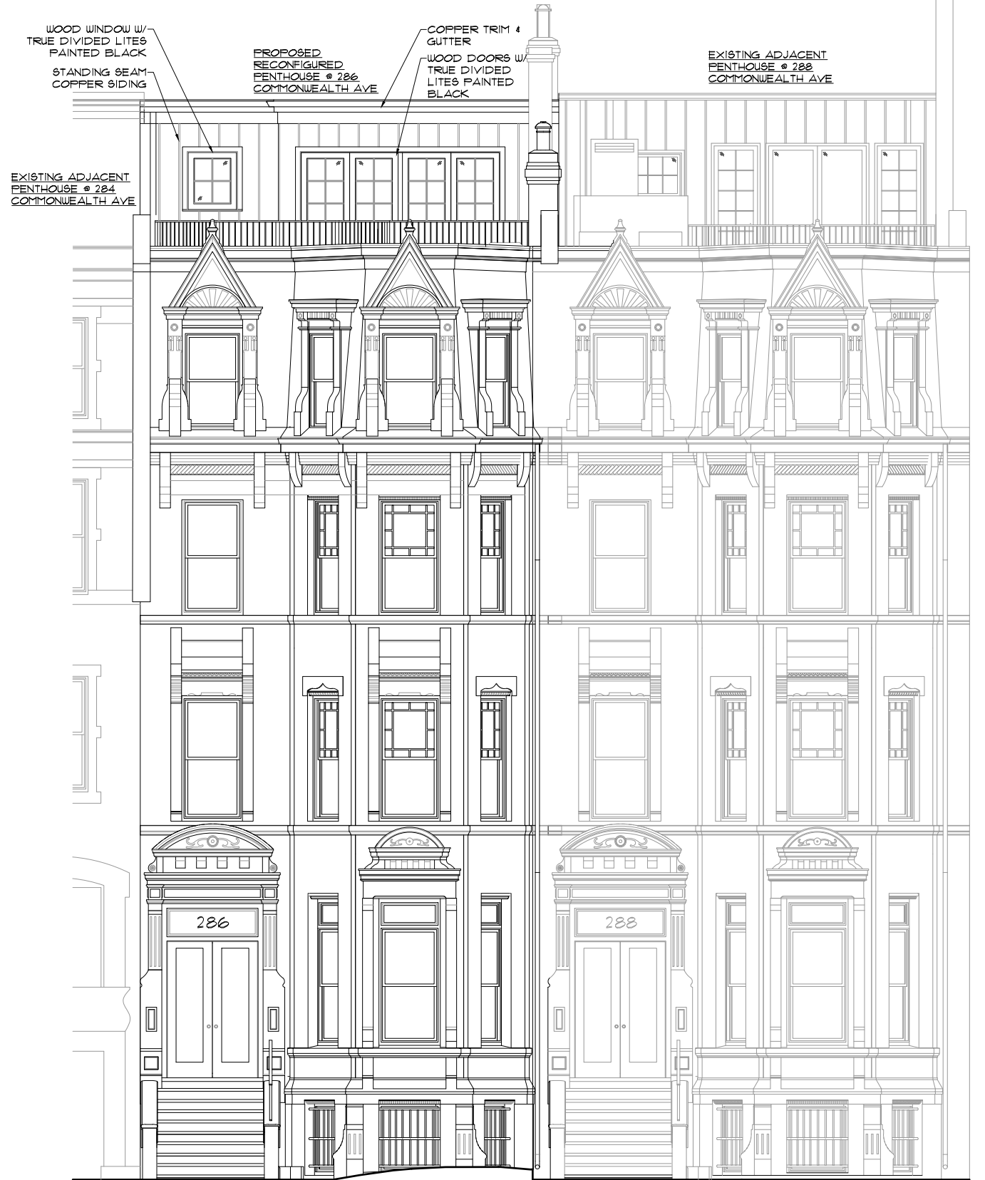
(P) PROPOSED FRONT ELEVATION FULL: 1/4" = 1'-0", HALF: 1/8" = 1'-0"
