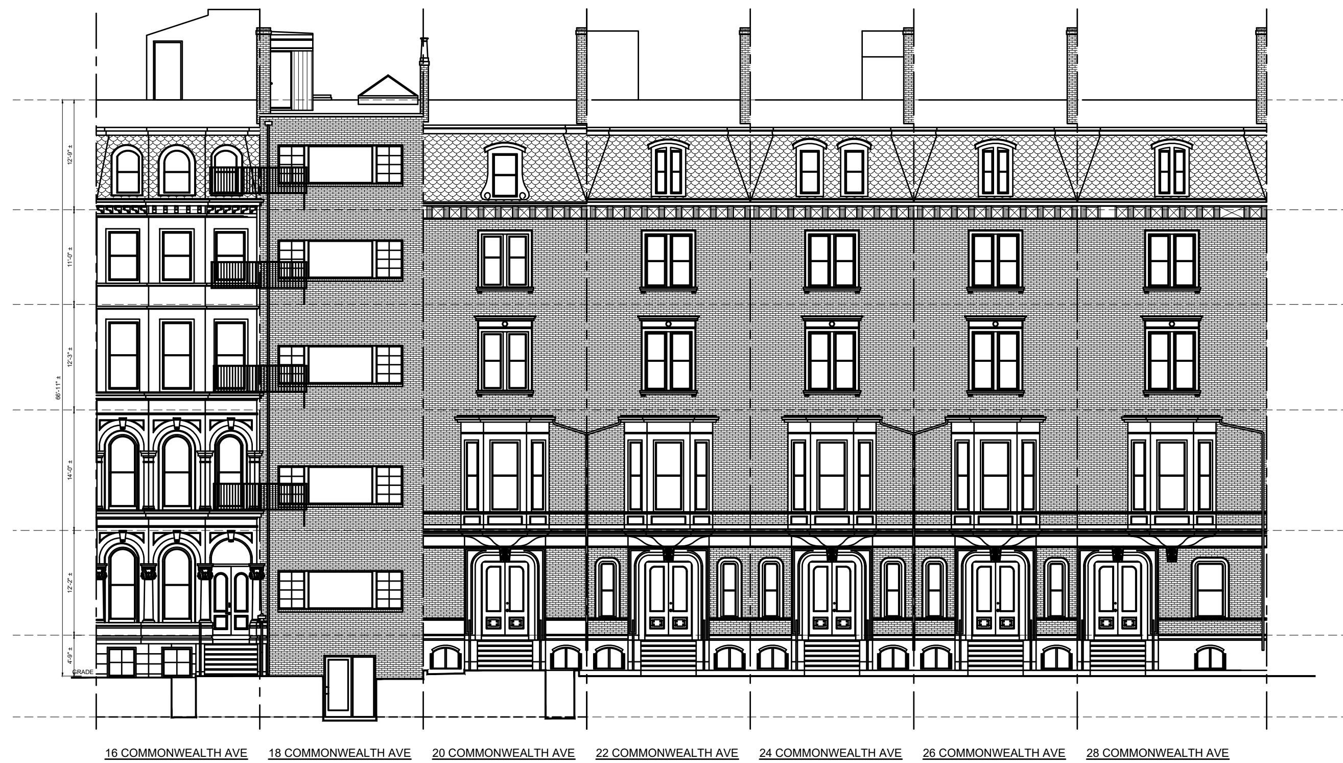
2 EXISTING FRONT ELEVATION 16-28 COMMONWEALTH AVENUE 3/32" = 1'-0"
