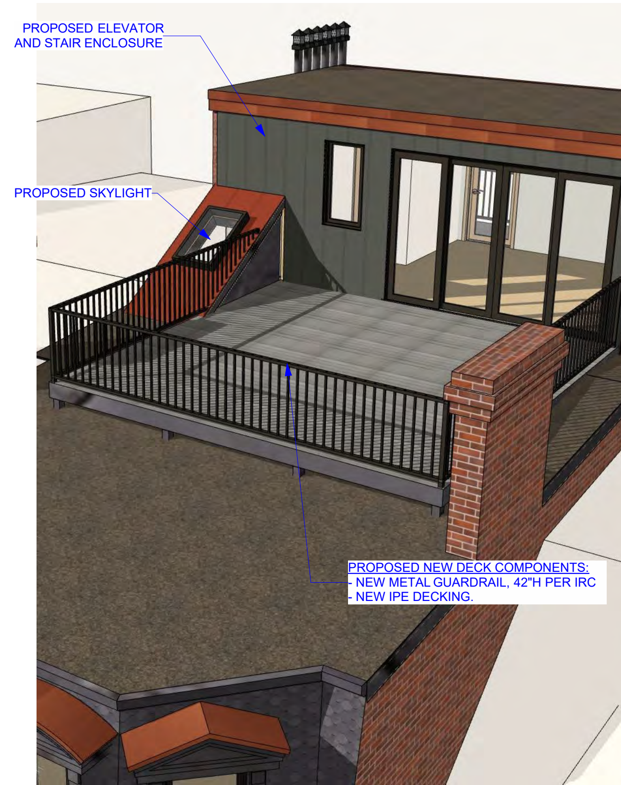
2A PROPOSED ROOF DECK & STAIR ENCLOSURE
