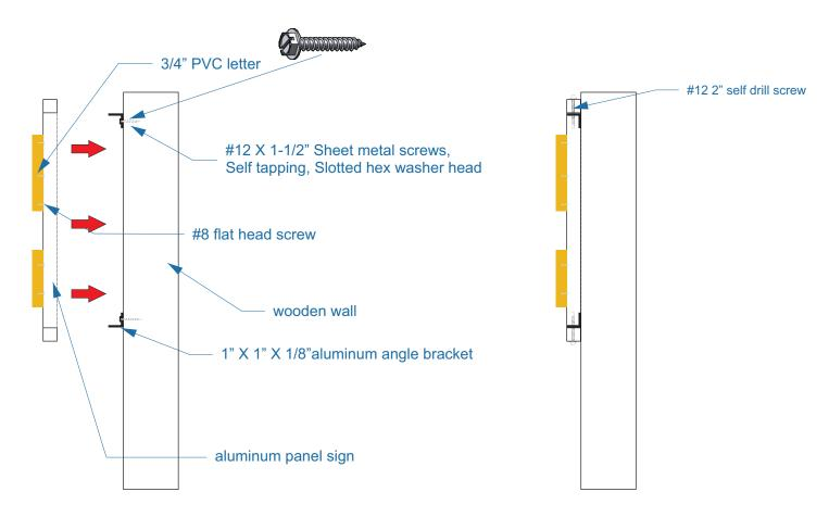
Each panel sign will be hold by 10 brackets, each bracket will needs to drill 1 hole to the wall for screw
