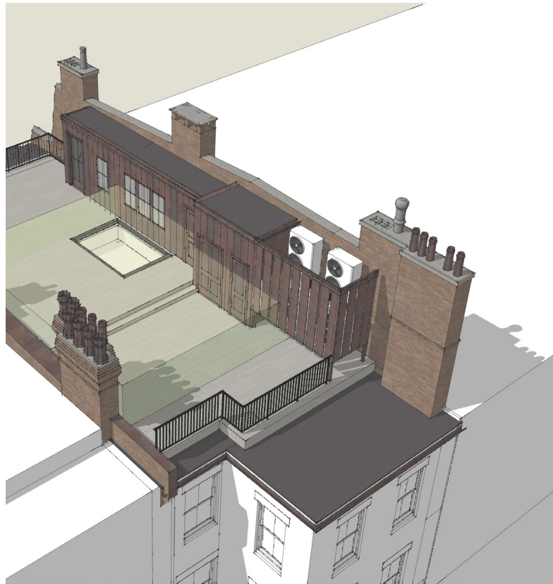
OPTION 1 (PREFERRED) 4 UNITS STACKED WITHIN COPPER ENCLOSURE
