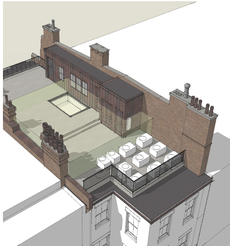
EXISTING ROOFTOP CONDITIONS 10 EXISTING HVAC UNITS
