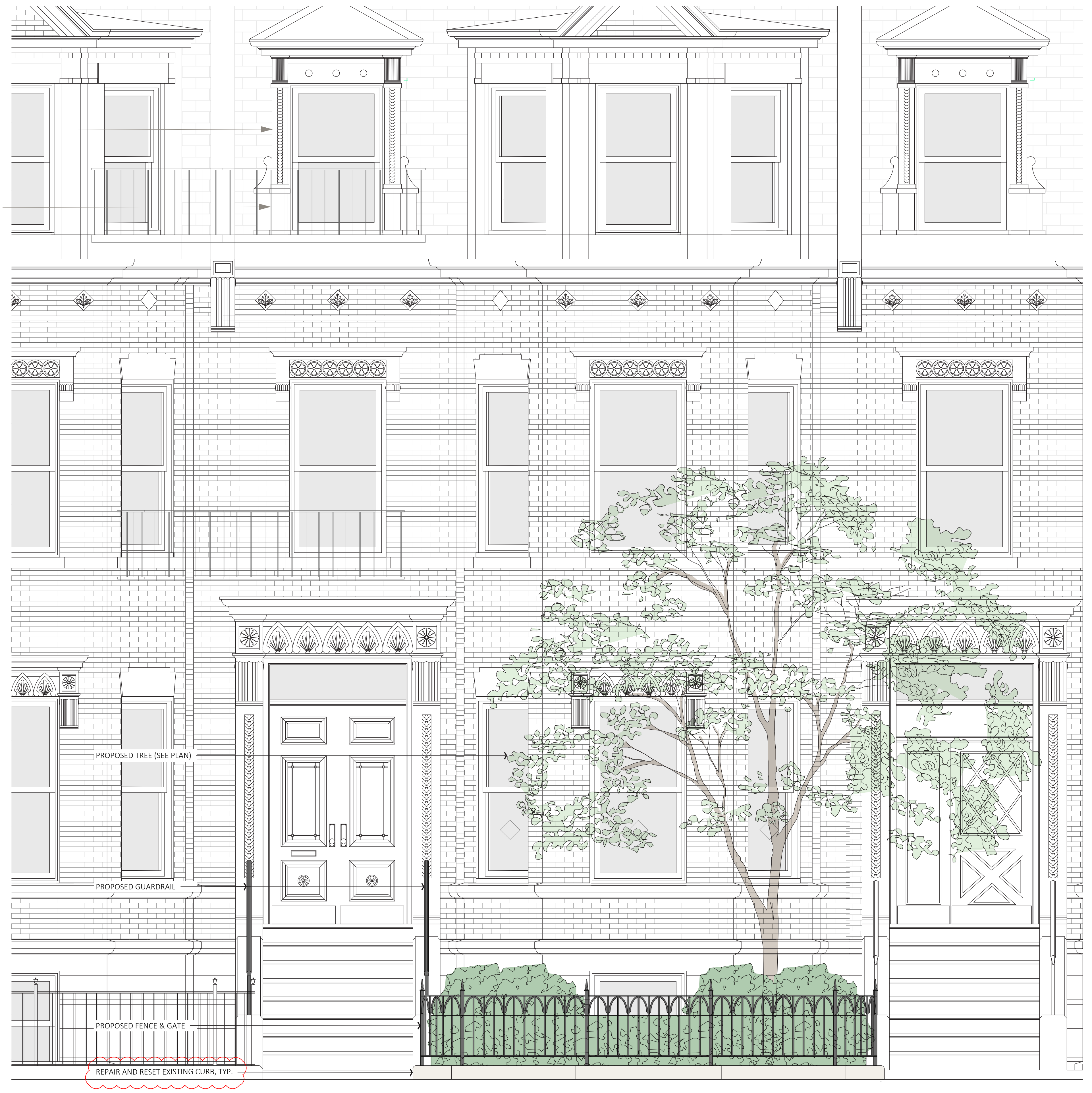
2 SECTION ELEVATION - LOOKING NORTH SCALE: 1/2" = 1'-0"
