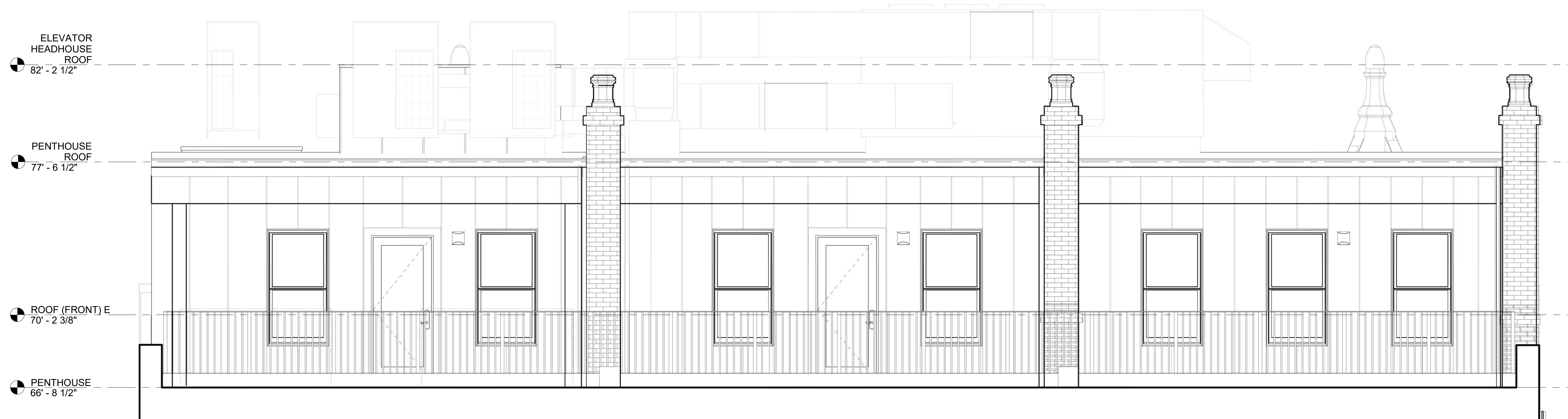
2 ENLARGED SOUTH ELEVATION - PENTHOUSE 3/8" = 1'-0"
