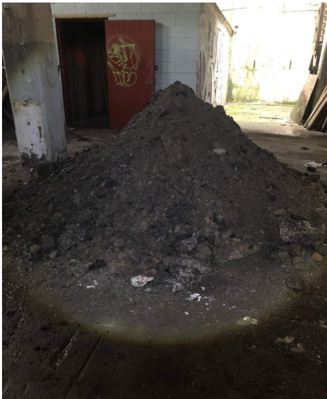
Photograph No. 7: Excavated material from test pit.
