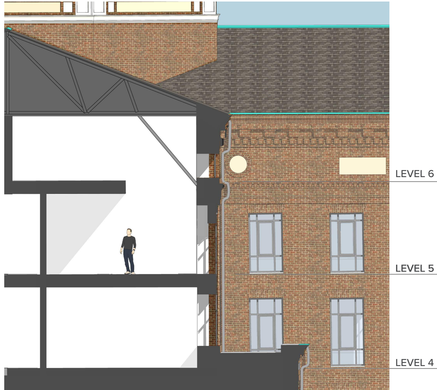
CLERESTORY WINDOW IN LEVEL 5 LOFT UNITS
