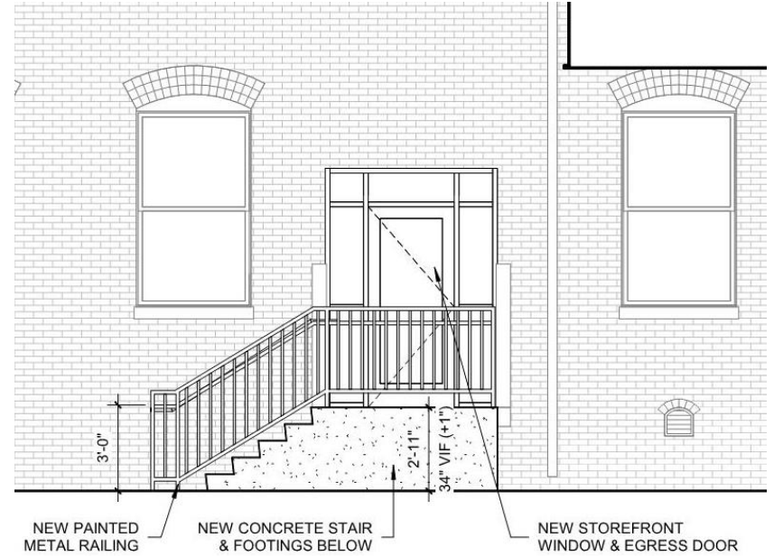
1 VIEW OF STAIR RAILING
