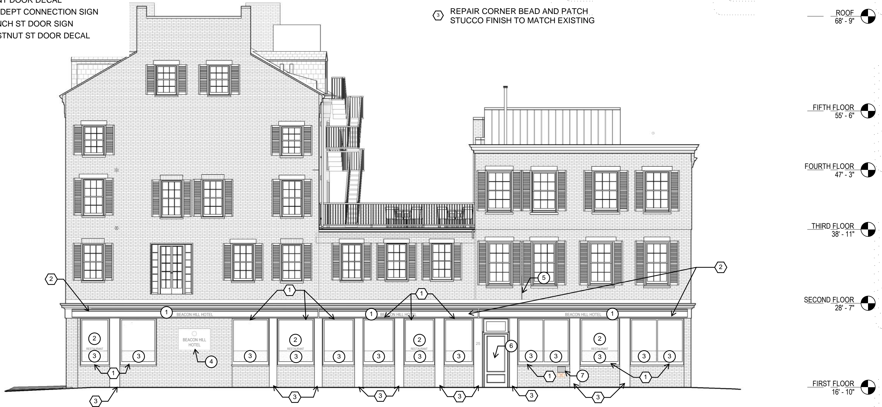
1 Charles St Elevation - Signage Locations 1/8" = 1'-0"
