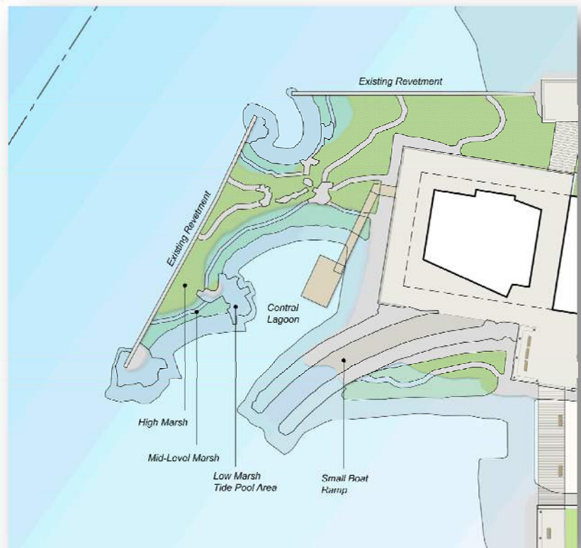
Figure 1: Proposed living shoreline at Clippership Wharf showing various planting terraces and salt marsh areas.
