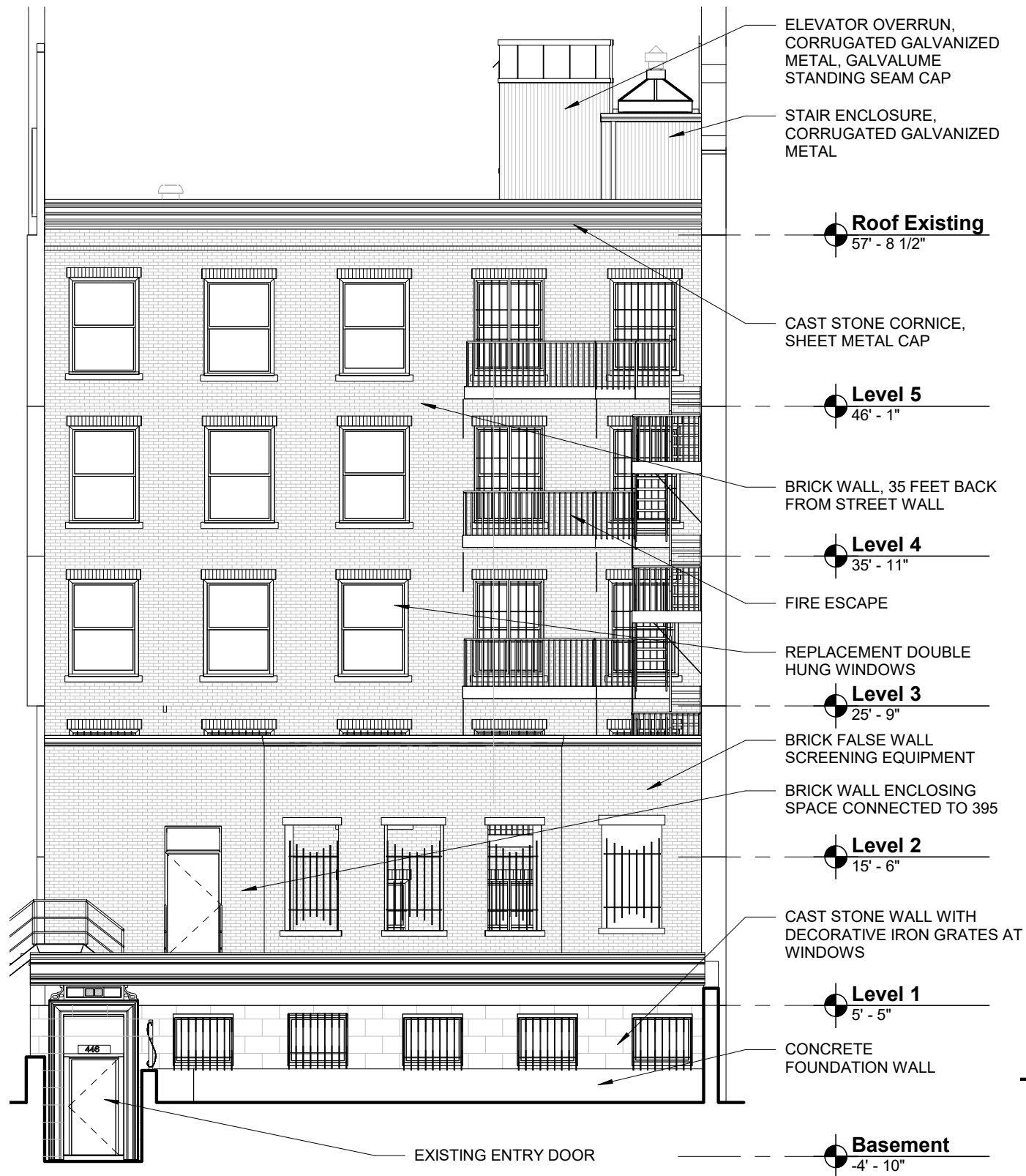
Marlborough Existing Elevation
