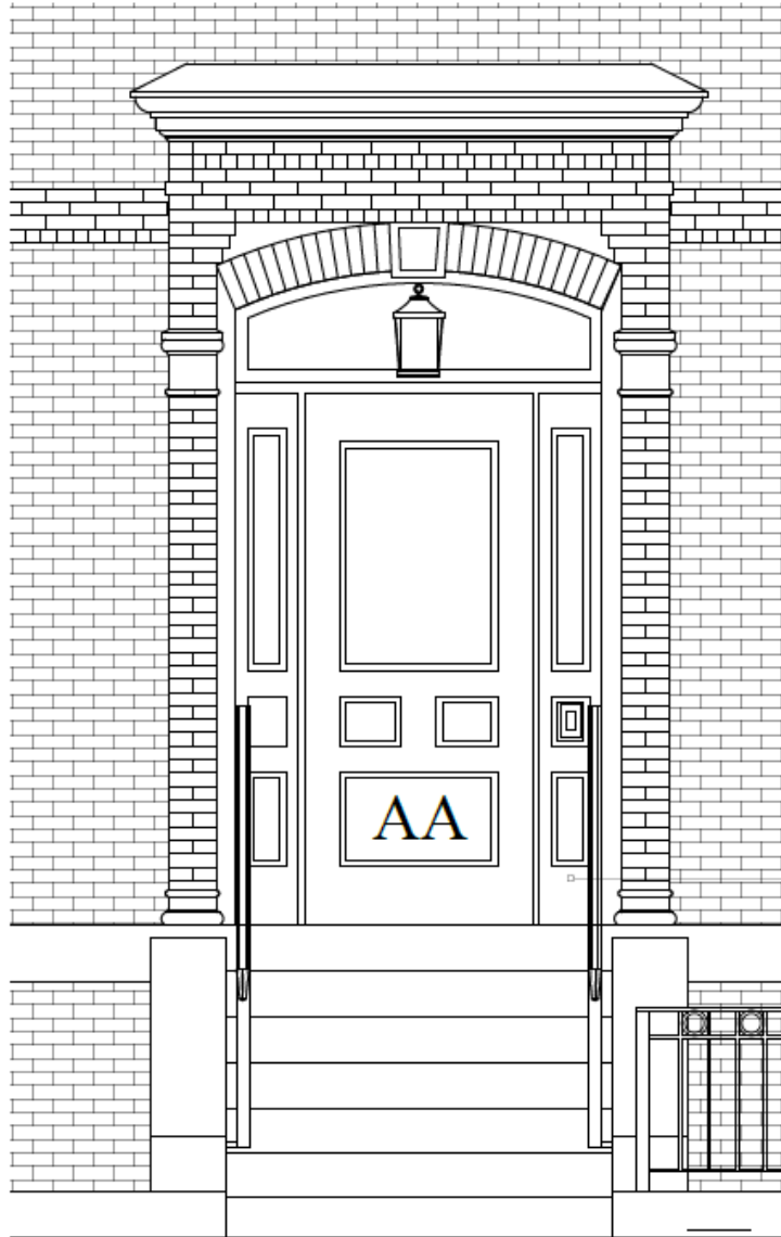
3 PROPOSED FRONT DOOR ELEVATION W/ INTERCOM 1/2" = 1'-0"
