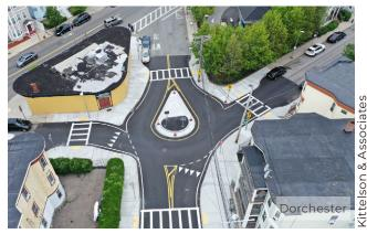
A small roundabout with a mountable central island that aids in directing vehicle traffic, slowing driving speeds, and facilitating safe pedestrian crossings.
