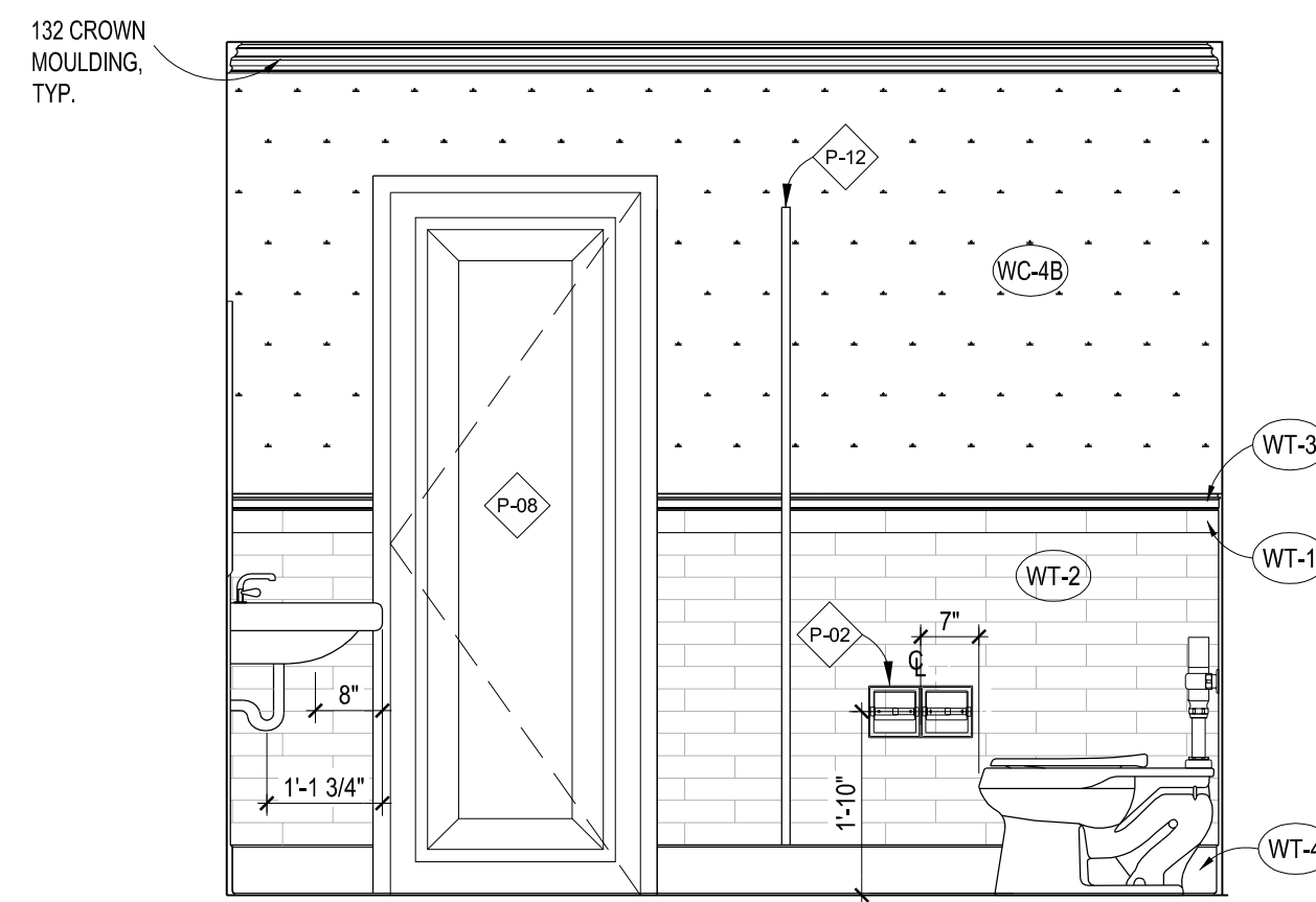
9 RESTROOM ELEVATION SCALE: 1/2"=1'-0"
