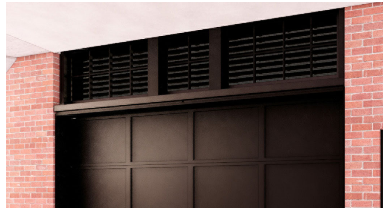
PROPOSED CLERESTORY WINDOW WITH LOUVER INSTALLATION BEHIND
