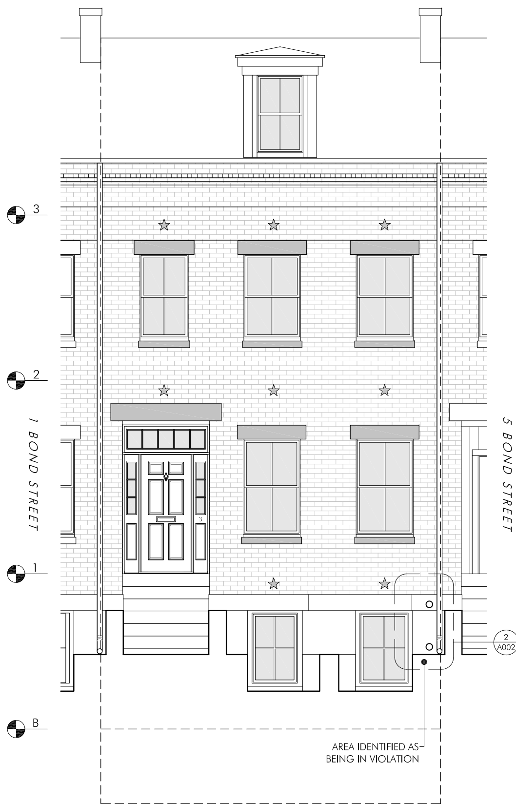
1 EXISTING EXTERIOR ELEVATION - FRONT SCALE: 3/16" = 1'-0"
