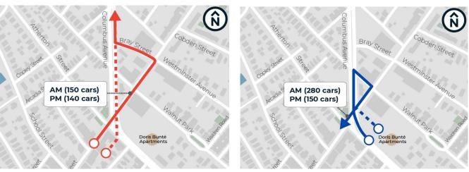
Existing/Option 1 - traffic flow for left-turning vehicles Option 2 - traffic flow for left-turning vehicles
