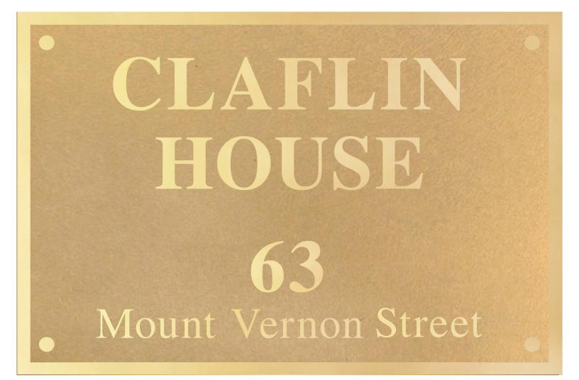
SPECS Cast Bronze, Alloy 922 Size: 12" x 8" Thickness: Approx. 5/16" Border: Single Line- .25"wide Background: Matte Finish Text and Border: Polished Finish Mounting: Four Pcs. #10 x 1.5" Oval Head Woodscrews painted to match background
