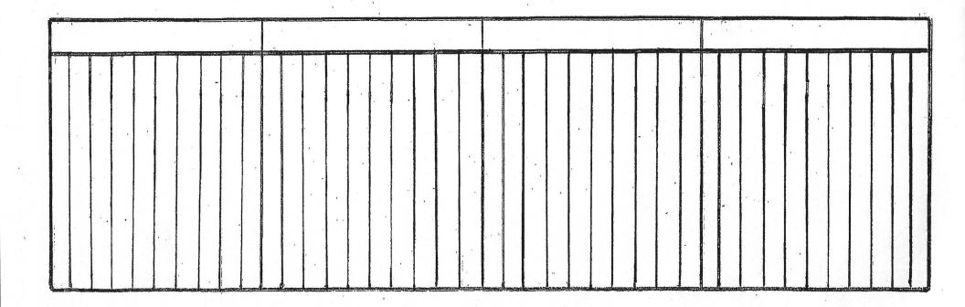
DIMENSIONS: 6 FEET HIGH BY 22 FEET LONG 8 INCH HORIZONTAL HEADER 5 FOOT 3INCH VERTICAL BOARD BASE
