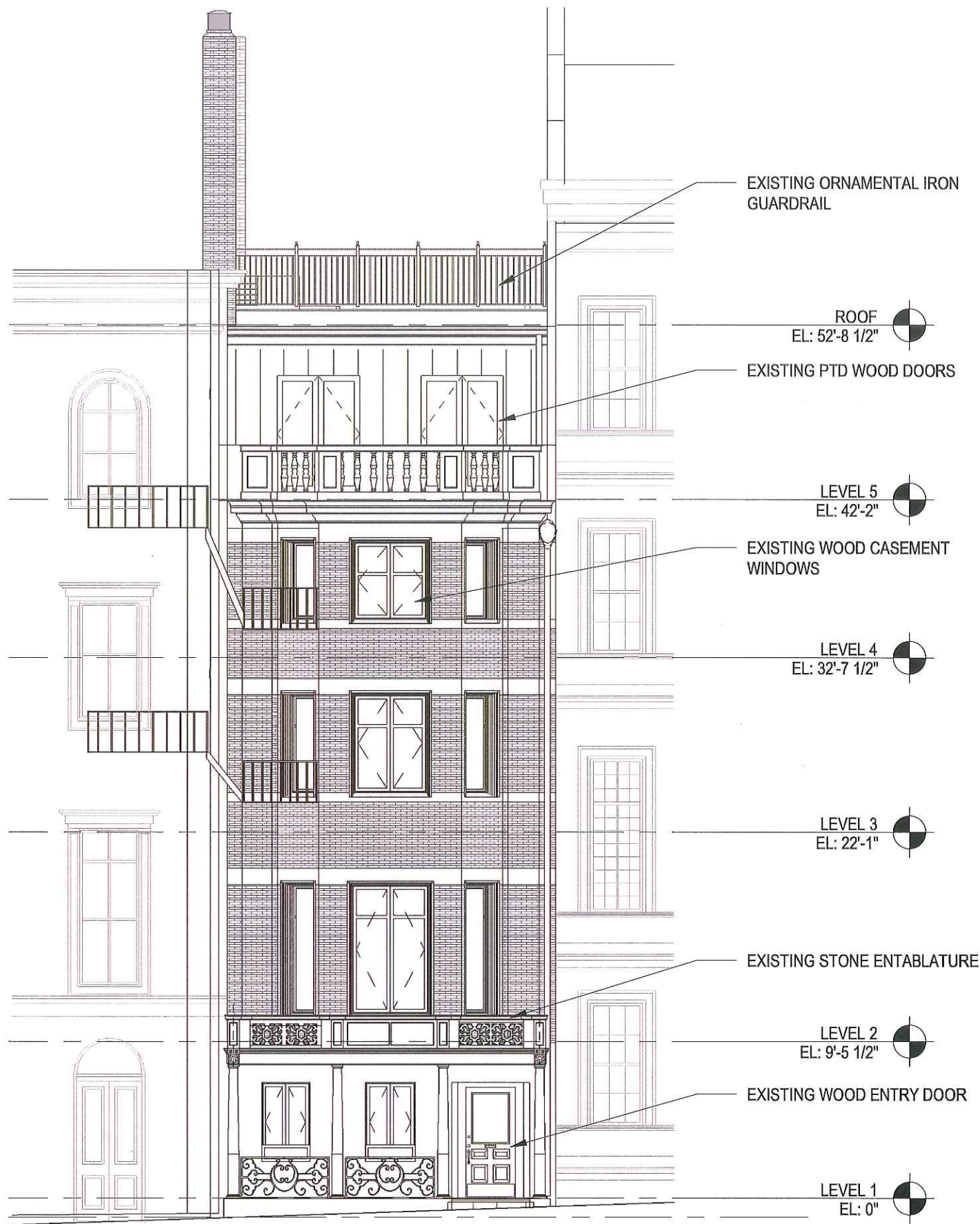
2 BEACON ST-EXISTING ELEVATION SCALE: 1/8" = 1'-0"
