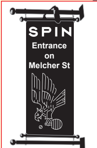
SUMMER STREET-Directional banner 72"x24" Vertical black Sunbrella banner on lit steel brackets
