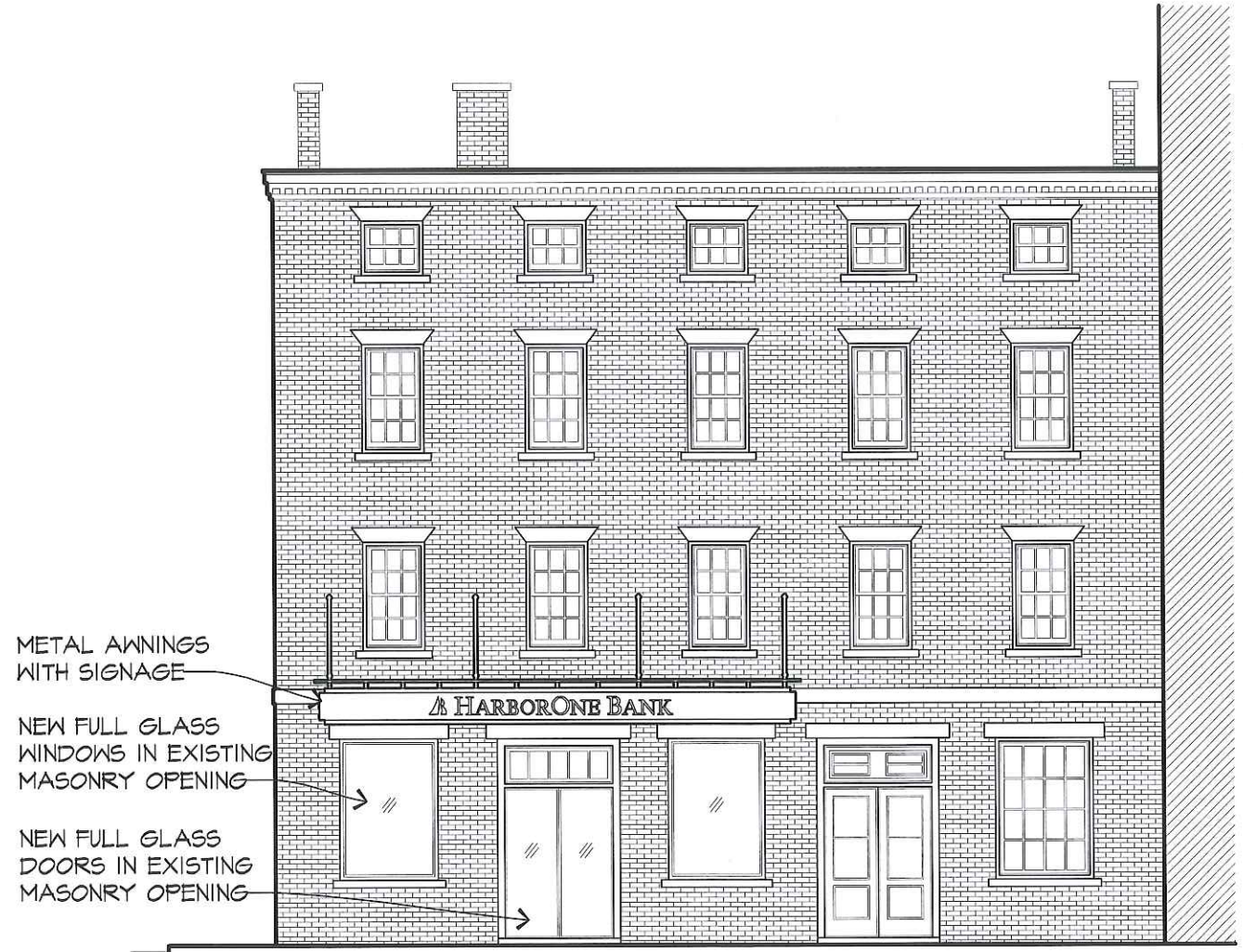
2 PROPOSED EAST ELEVATION SCALE: 1/8" = 1'-0"
