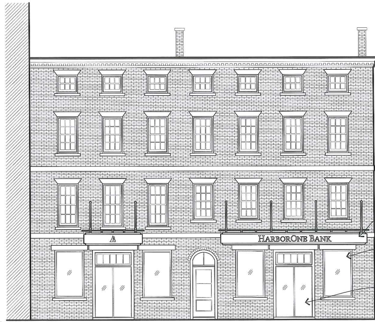
2 PROPOSED SOUTH ELEVATION SCALE: 1/8" = 1'-0"
