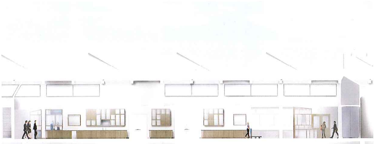
Section of Sawtooth skylights with diffused north light
