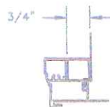
CLAD BRICKMOULD CASING WITH OPTIONAL J-CHANNEL COVER
