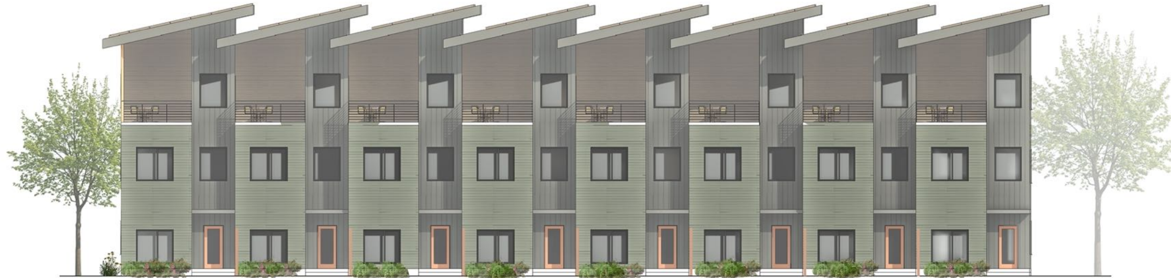
② ROWHOUSE EAST ELEVATION 1/16" = 1'-0"
